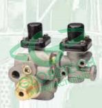
Body height: 5-3/4" Delivery ports: (4) 3/8" PT Reservoir charging ports: (2) 1/4" PT Trailer supply ports: (1) 1/4" PT Trailer service ports: (1) 1/4" PT Reservoir connection: (1) GTA-101112
